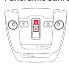
The sunroof operation is controlled through a multidirectional switch. The ignition or Engine Start/Stop button needs to be in the ON position to operate the sunroof.
