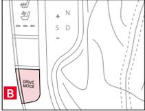
Drive modes **A**: NORMAL, SPORT, and SMART are available for vehicle operator selection, based on preference, and travel conditions. Mode selection simply requires the press of the DRIVE MODE button **B**, and will display selection on the Instrument Cluster.
